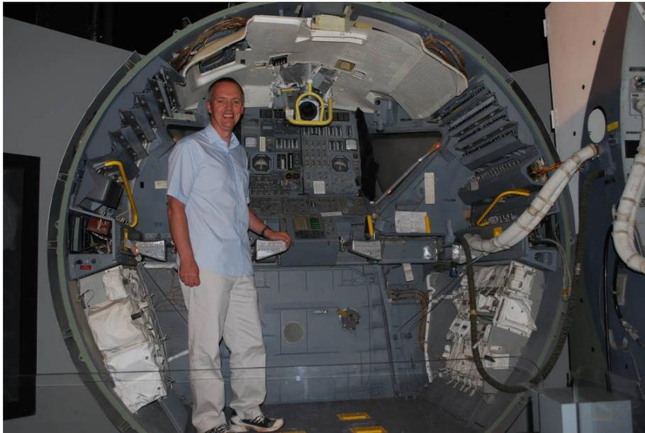
**Front half of LM simulator used by astronauts for training.**
